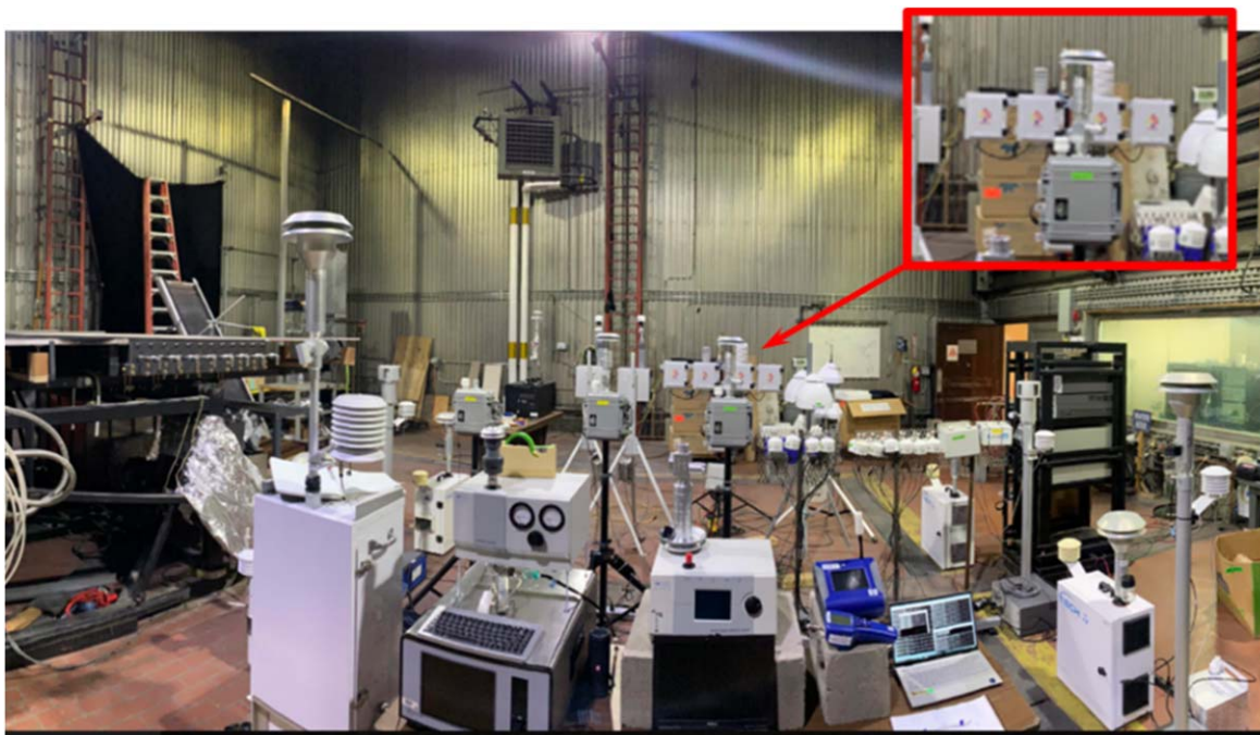
Figure 11. Thingy: AQ monitors with SPEC Sensor gas sensors and Sensirion PM and CO 2 sensors, as specified by KWJ following laboratory evaluations.
